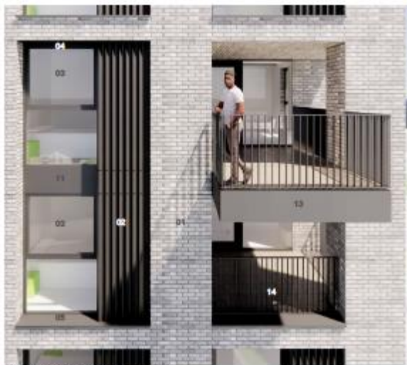
West Facade Recessed & Projecting Balcony
